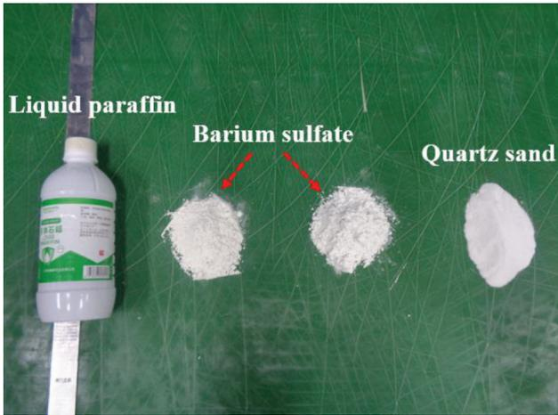
Fig. 4 Base friction model test material formulation
