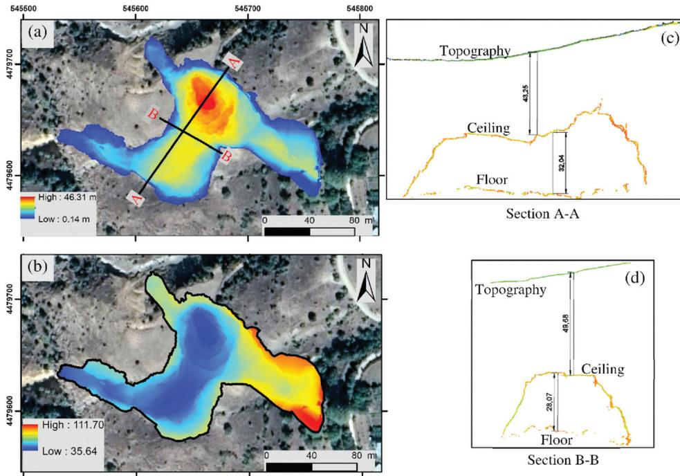
**Fig. 8** UAV and TLS elevation models of the Akcakale cave and data generated from the integrated point clouds: (a) ceiling height, (b) depth from surface, (c, d) sample sections including cave and surface topography
