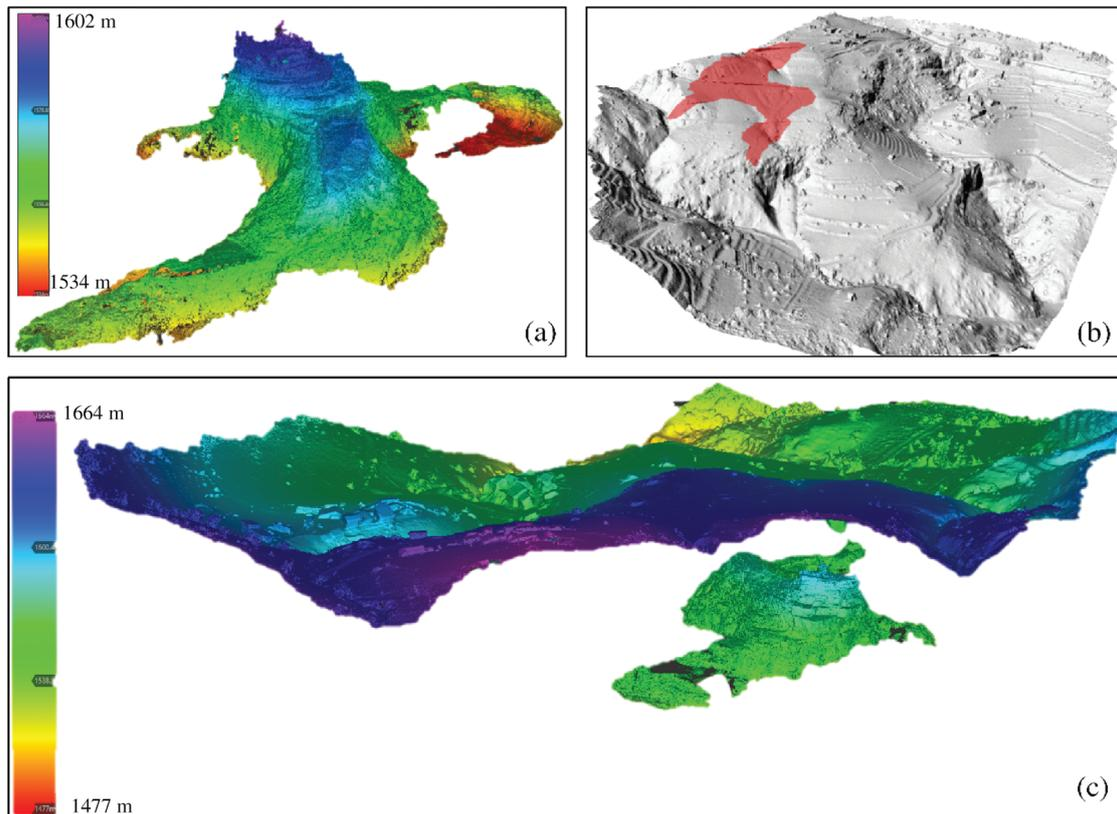
**Fig. 6** Examples of the data obtained using TLS and UAV systems: (a) the Akcakale Cave TLS point cloud; (b) 3D representation of the cave projection on the hillshade generated from DSM; (c) integration of the UAV and TLS point clouds
