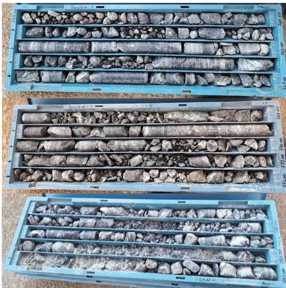
Fig. 7 Cores were taken from 757–782 m depths, where water pressure tests were performed in borehole SK-4 (every section dimension of boxes is standardly 100 cm, and there are 5 sections in a core box)
