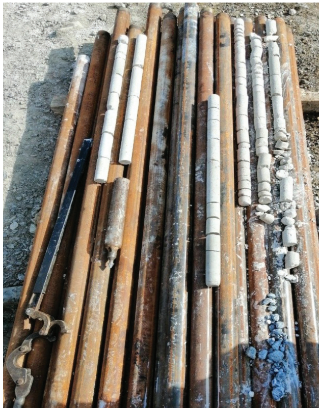
Fig. 6 Cement cores taken from the borehole with the wireline drilling equipment for controlling the grouting operation
