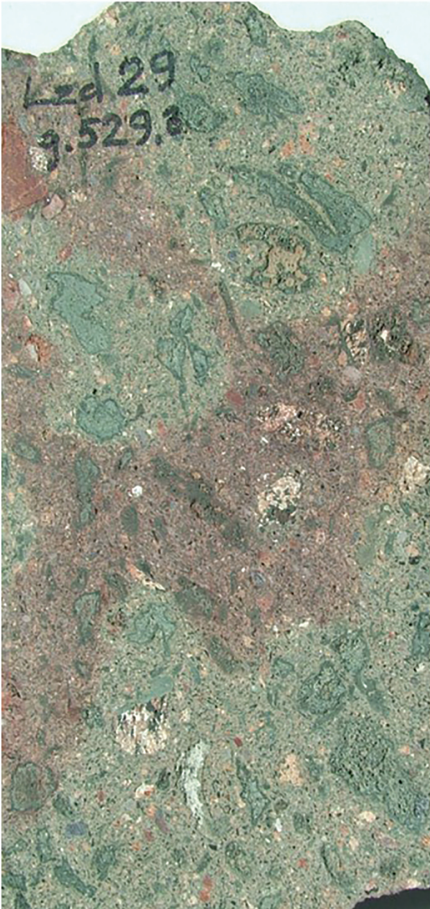
Fig. 8 Drill core of suevite: green inclusions – altered (chloritised?) glassy material; borehole Lzd-29/529.3 m; the diameter of drill core – 5 cm
