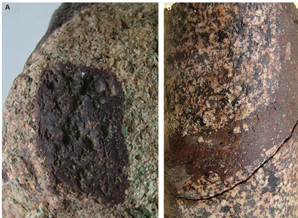
Fig. 10 Impact melt rocks: A – fragments of the impact melt rock in the sandstone of the sedimentary fill of the crater, size – 3 × 4 centimetres; borehole D-1422/352.5 m; B – granodiorite, with veins of impact glass; borehole D-1422/373.2 m; the diameter of drill core – 5 cm
