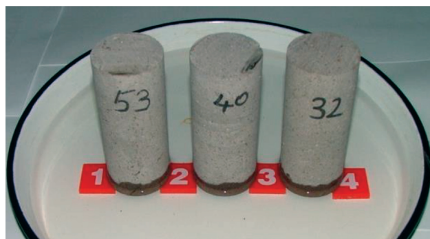
Fig. 7 Capillary water rise experiment of andesite samples
