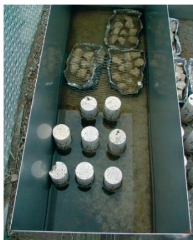
Fig. 8 View of travertine samples kept in the undrained section of the investigation tank at the Afyon Meteorological Station
