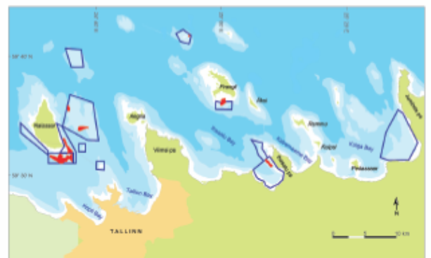
Fig. 5. Sand investigation areas (blue polygons) and approved resources of subbottom sand (red polygons) in the surroundings of Tallinn.
