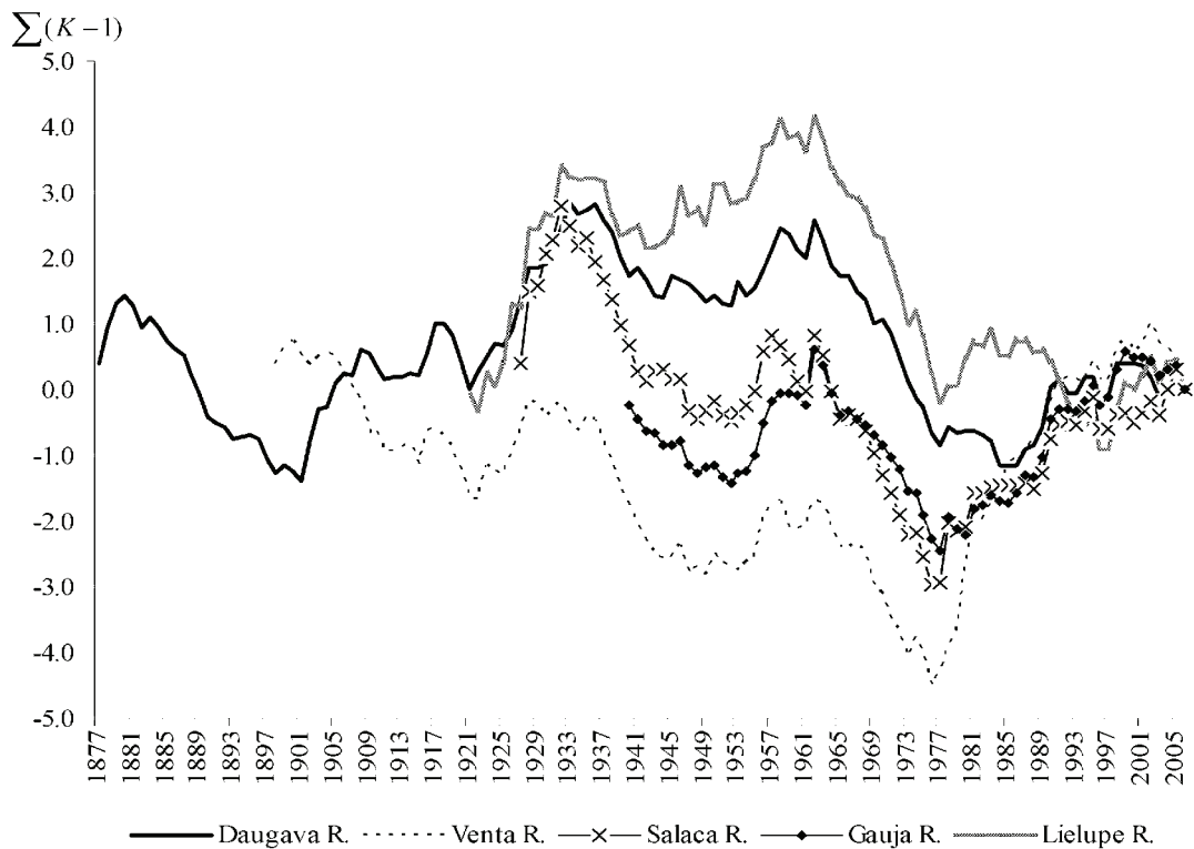
Fig. 7. Normalized integral curves for coefficients of the annual runoffs of rivers in Latvia.
