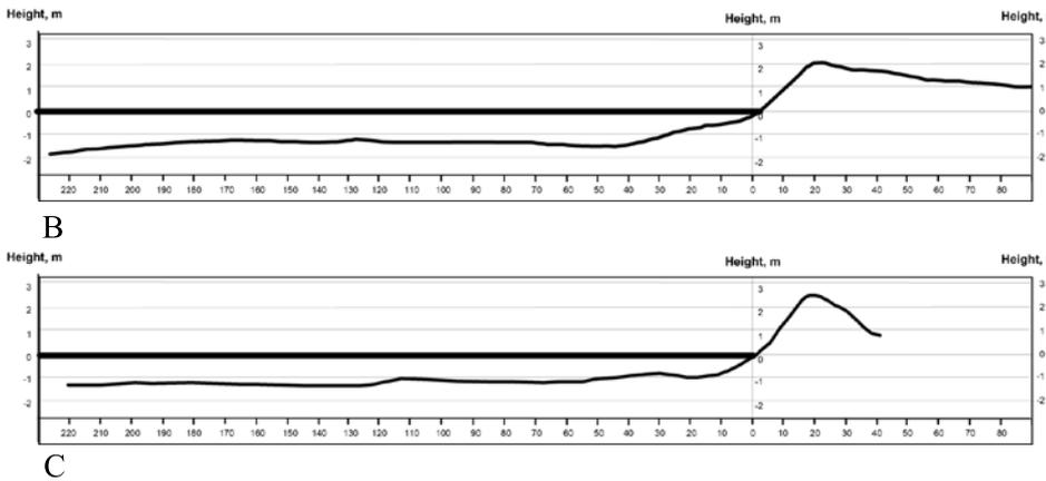
Fig. 5. Alternation of erosion, transit and accretion areas in the vicinity of Bolshaya Izhora village (A) and coastal profiles of accretion (B) and erosion (C) zones (II in Fig. 1).
