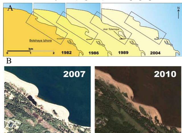
Fig. 7. Formation of connected spits: A – 500 m long sand body to the west of the Tchernaya River mouth; B – transformation of long-shore sand waves into connected spits (2007–2010).
