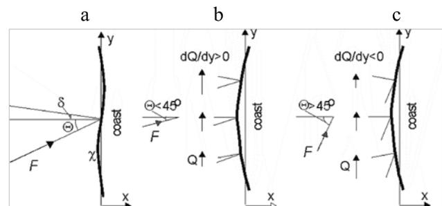
Fig. 11. (a) – definition sketch; (b) and (c) – changes in sediment flux in cases of small (b) and large (c) angles of wave approach to the coast.
