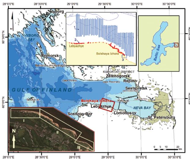
Fig. 1. The study area (red rectangle) in the eastern Gulf of Finland. 1 – side-scan and echo sounding profiles; 2 – off-shore sampling stations; 3 – area of geo-radar study. I – III – coastal segments with different dynamics.
