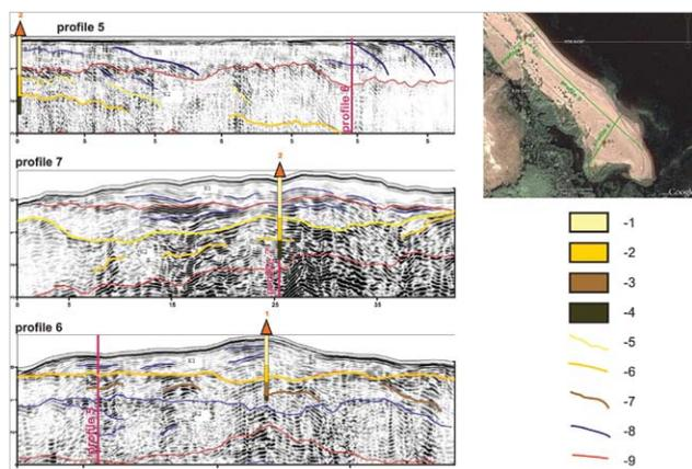
Fig. 8. Geo-radar profiles of the distal part of the spit. 1 – coarse-grained poorly sorted sands; 2 – fine-grained medium sorted sands; 3 – coarse-grained sands with pebbles and gravel; 4 – clayey black mud with remains of plants; 5 – 7 – geophysical boundaries confirmed by drilling; 8 – 9 – geophysical boundaries.
