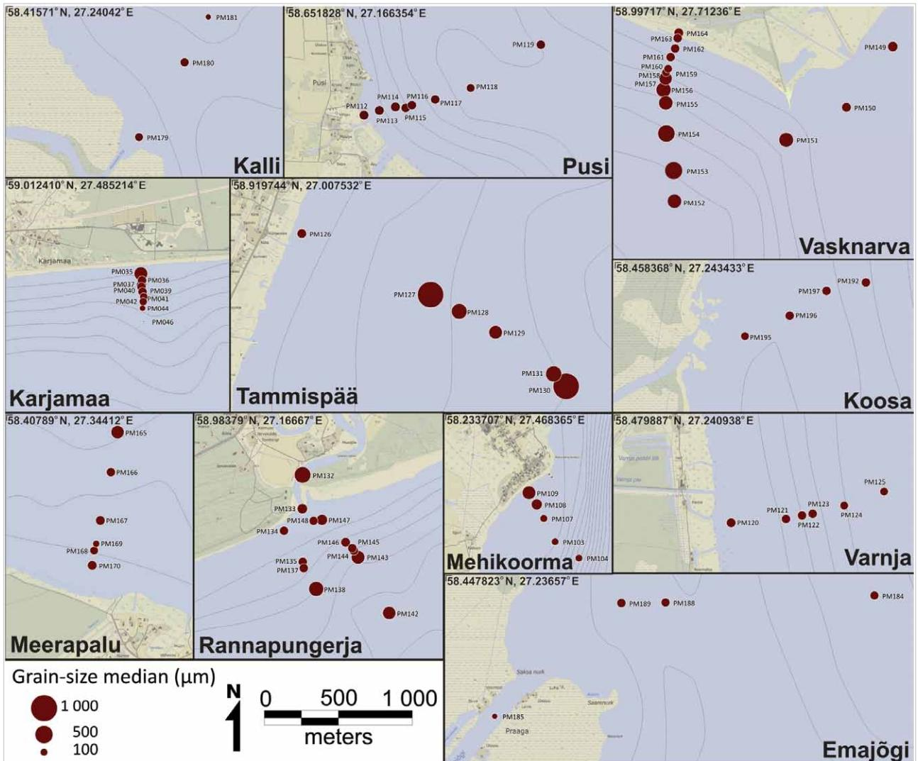
**Fig. 4** Grain size median values of sampling points on studied sites. Dashed lines show the water depth with 1 m step. Compiled by J. Terasmaa, 2013.
