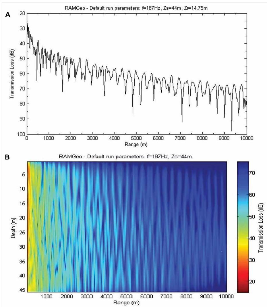
**Fig. 4** **A.** Range dependant noise transmission loss. **B.** Range and depth dependant noise transmission loss (azimuthal direction from South to North).
