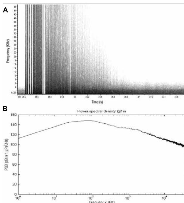
**Fig. 3 A.** Underwater noise spectra. **B.** Power spectral density on a logarithmic scale (24 kg TNT explosion).
