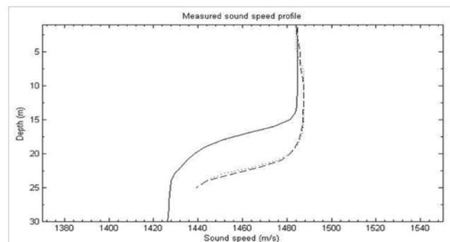
**Fig. 2** SSP measured in the Lithuanian Baltic Sea area: even line measured on 22 August, dashed line on 25 August and dotted line on 26 August (NAVY 2013).
