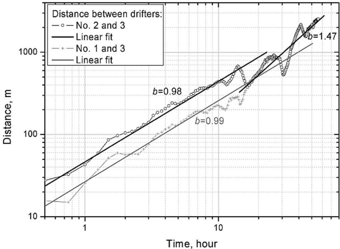
**Fig. 6** Time dependence of the distance between pairs of drifters in log-log scale. Compiled by L. Davulienė.
