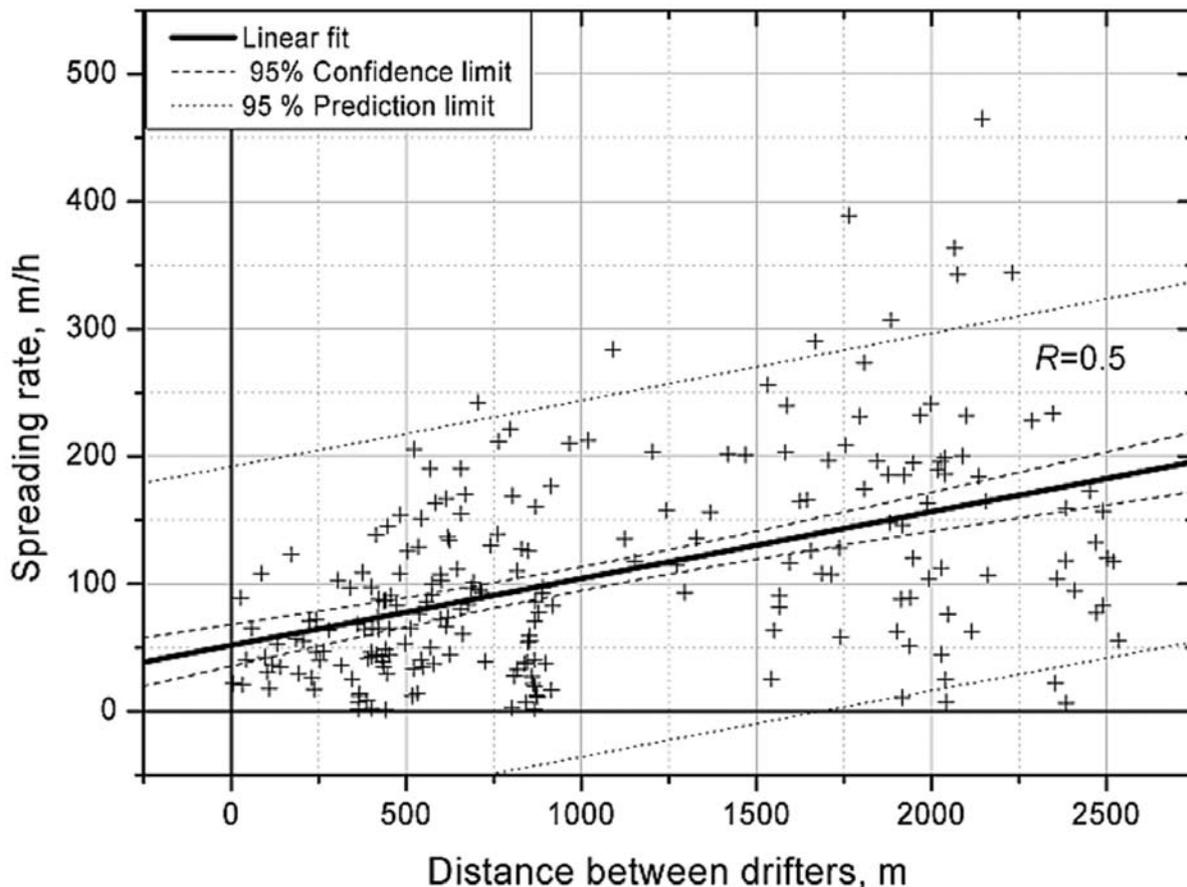
Fig. 5 Spreading rate dependence on the distance between drifters. Compiled by L. Davulienė.
