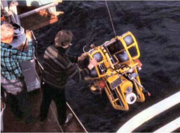
Fig. 6 The remotely operated underwater vehicle (ROV) constructed in 1967 at GTK being carefully deployed overboard by electronics engineer Leevi Koponen while geologist Esa Kukkonen is paying out the tether cable. The video camera is used for navigation and general observation (yellow casing) and the still camera (white casing) located low on the vehicle to allow good quality photography even in very poor visibility
