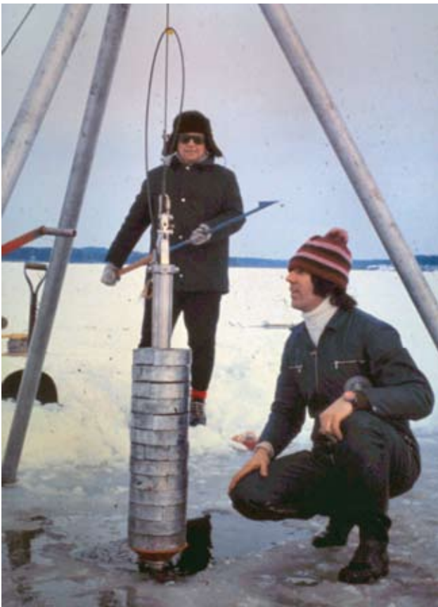
Fig. 7 Although the piston corer was originally designed for marine sediment sampling it is just as suitable for wintertime coring in deep lakes or even coastal lagoons not reachable by boat. Heikki Ignatius in the background with icepick in his hands although the hole in the ice was made with a long chainsaw. Technician Pauli Kaijola is checking the lead weights. Photo taken by B. Winterhalter 50 years ago in Finnish Lapland
