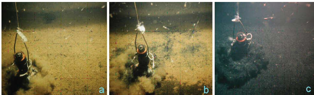
Fig. 5 Automatic sea floor camera images taken down a gentle slope from a drifting ship in the Fårö Deep, Northern Baltic Sea. The depth varies from 101 m (a), 102 m (b) and 109 m (c) showing from left to right increasing level of anoxia. Pictures like these are excellent indicators of the distribution of anoxia in this case loss of anoxia following a slow dissipation of oxygen and deposition of oxidized (brown) fluffy sediment from overlying waters (See Niemistö, Winterhalter 1977)
