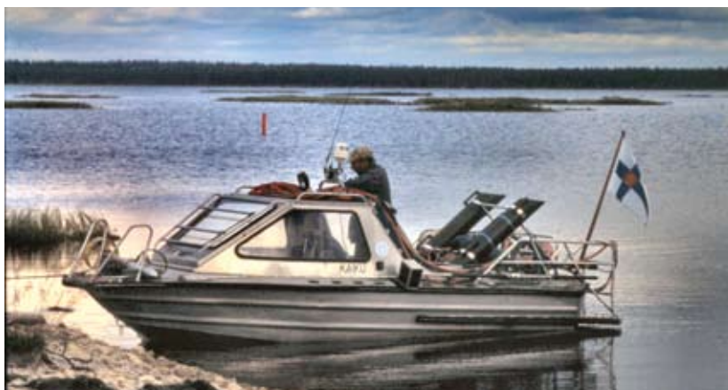
Fig. 12 The Kaiku (=Echo) motorboat was fully equipped with Meridata’s MDPS-integrated GPS-positioning, echo-sounder, side scan sonar and single channel low frequency towed profiler with hydrophone streamer for wide band acoustics with excellent penetration in sand, gravel and till. Electronics engineer Matti Tuhkanen is the main operator of the boat and its data acquisition equipment
