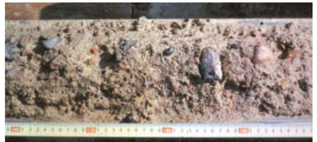
Fig. 10 Example of typical diamicton (till) sampled with the vibro-hammer corer (scale in centimeters)
