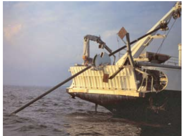
Fig. 9 (Above photo ) shows the retrieval of the 12 m long vibro-hammer corer for sampling sand and gravel under a sufficiently thick layer of silt or clay to keep the corer vertical. The attitude and penetration of the corer was controlled with an echosounder transducer located under the bow of Geola . On deck the plastic core liner was extracted, split, described and sub sampled
