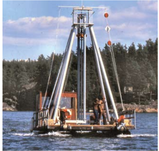
Fig. 8 Above photo of the first “vessel” built for rapid sand/gravel coring in the sheltered waters of our archipelago. The 6 m corer was lowered through the central “moon-pool” while twin anchors steadied the operation. The actual site was chosen based on previous acoustic profiling
