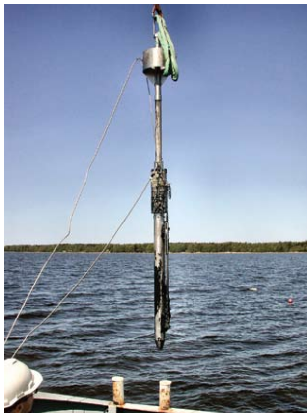
Fig. 15 The Söderberg gas-corer being used on Geola for sampling gas-charged sediments near the Olkiluoto nuclear power plant
