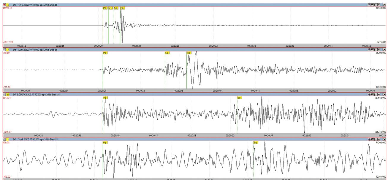
**Fig. 11** Records of the vertical component of VYB, IZM, LOPUX, VAL stations (top-down, respectively) filtered in the 2–8 Hz band (Butterworth, 3rd order) of the event of 18.12.2016 at 00:20 with  $M_L$  2.1. The records are aligned for the first arrival of Pg
