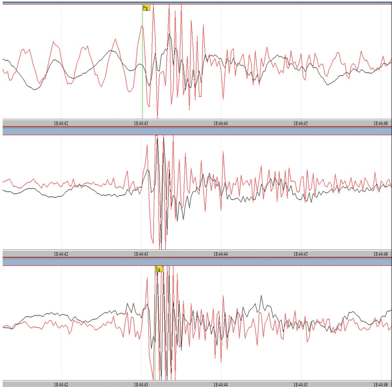
**Fig. 8** Recording of the ground movement velocity in  $\mu\text{m/s}$  of the Valaam seismic station (VAL) during the earthquake on 31 July 2010 at 18:44 GMT (the components of the top-down recording are Z, EW, NS)
