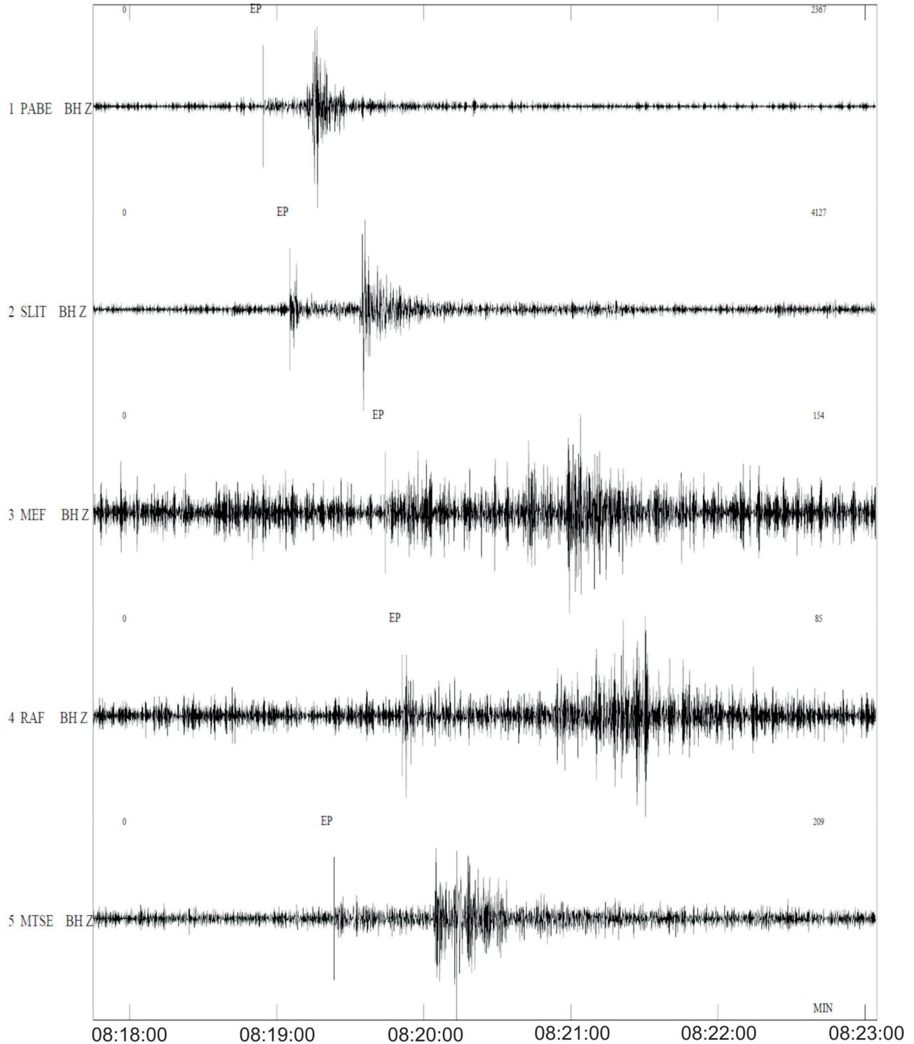
**Fig. 5** Records of seismic event with signs of an earthquake near the Curonian Lagoon (Lithuania) on 12 June 2015. Notes: filtering 3.0–8.0 Hz; only the Z-components are shown
