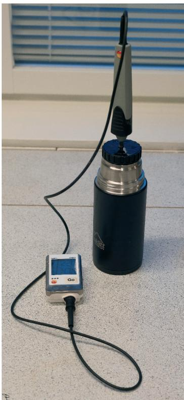
**Fig. 6** Photo showing a simple “calorimeter” consisting of a steel thermos and temperature sensor. Photo: Per Lindh
