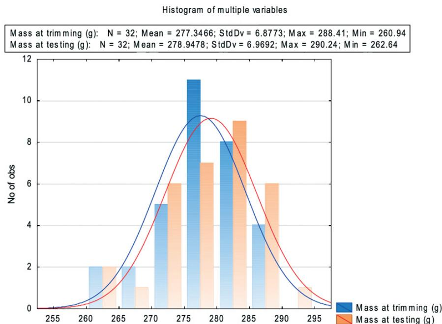
Fig. 4 Graph showing the weight of the samples immediately after trimming and before compression
