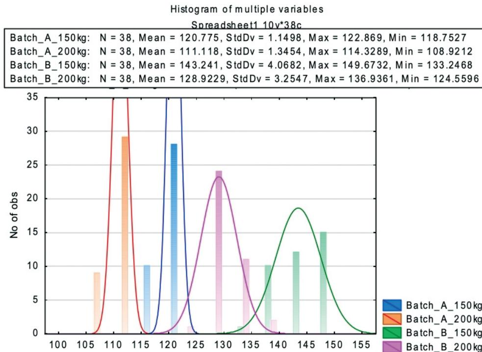
**Fig. 5** Ratio of water to binder determined when trimming samples included in the factor experiment
