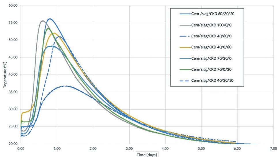
**Fig. 7** Reactivity test to evaluate the variations in temperature in a slurry with water binder number (VBT) of 1.0 and various binder ratios (proportions of Portland cement/slag/CKD)
