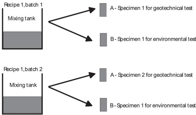
**Fig. 2** Schematic figure showing how the number of admixtures can be reduced while maintaining the functionality in terms of the true duplicate tests for geotechnical and environmental geotechnical test samples performed in the Swedish Geotechnical Institute (SGI)
