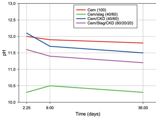
**Fig. 8** The pH variations over time for the four tested specimens with varied ratios of Portland cement/slag/CKD
