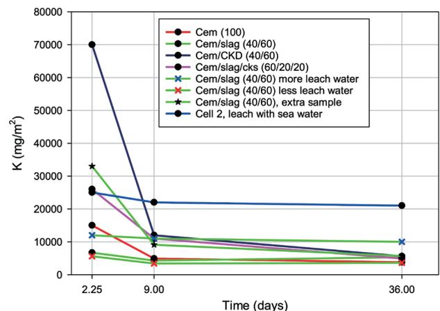
**Fig. 11** Leaching of potassium (K) in the experiments with different recipes and changed water conditions, and leaching from Cell 2 reported in the pilot experiment for comparison
