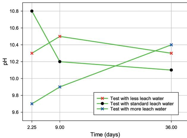
**Fig. 9** The pH variations over time in surface leaching experiments where the amount of water changed
