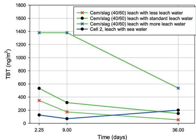
**Fig. 10** Leaching of TBT from seawater according to the standard experiments by different water and binder ratios (Portland cement/slag/CKD) and leaching of TBT
