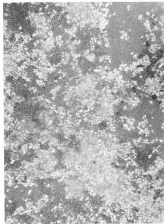
Fig. 2a Chomogenic-diagenetic manganese carbonates of the Gotland basin muds (station 3173, R/V „Professor Dobrynin“, depth 243 m., horizon 145—150 cm) — a general aspect of the carbonates (white) in a smear under the polarizing microscope. Nicols x, increasing 250. Black oval grains — iron sulphides.
