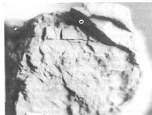
Fig. 6. Middle Pleistocene intertill clay: note the disturbed primary bedded texture. SD 25.6 m, magn. 2.5 X.
