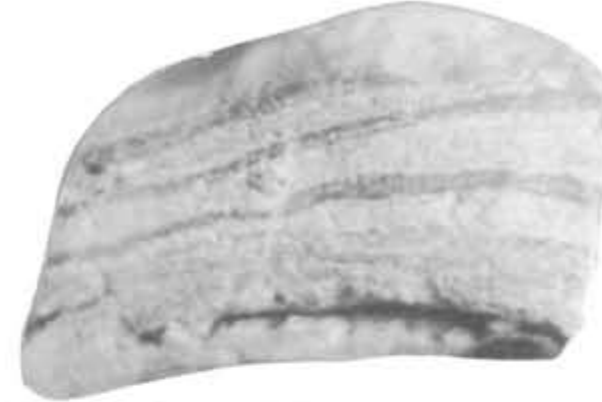
Fig. 4. Upper Pleistocene glaciolacustrine varved clay. Clay (dark) and sandy-silt (light) with gravel-size grains laminae are alternating. SD 0.1 m, magn. 3 X.
